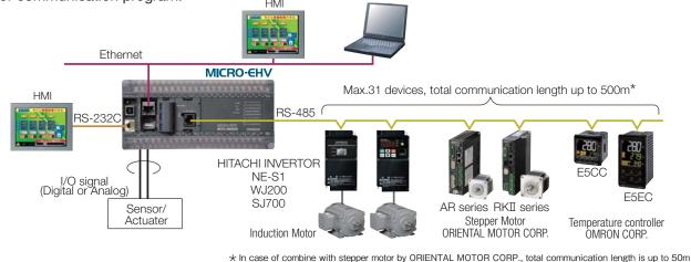
Connection only communication line to the slave device. It's "omit wiring" and "smart control".
