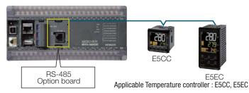
"OCTP1" command is dedicated command of control and monitoring for OMRON's temperature controller. (Applicable temperature controller : E5CC, E5EC)
